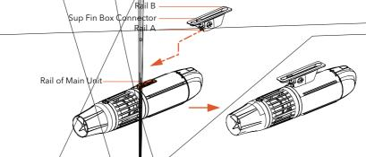
Step 2: Take one locating pin, align with hole A, and insert for locking.
