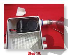
Assemble the hose to the outlet and attach a metallic clamp if needed. Put the filtration net back to position and screw back the acrylic lid.
