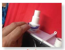
Step 9: Insert the Outlet and Fix the blue Clamp. Note that the Clamp must be inserted fully inside the referring sockets of the adapter.
