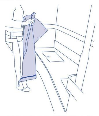
2 Place the bunknet with silver side up. Check if final height of the bunknet is ok.
