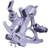
construction as the Mk15, but with the differences. The 'all-view' following mirror (which Davis call the Beam Converger) gives a full-width horizon with the heavenly body superimposed on it, so there's no left & right side. Many people find this easier to use than a 'split-view'.
